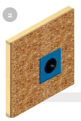
**Optional:** Using noncorrosive fasteners, secure the Quickflash® panel to the structure from the mid-point of the panel to the top.
