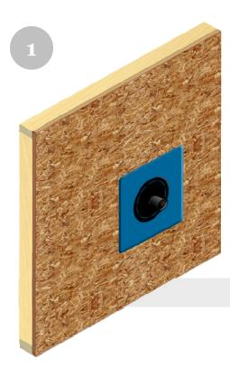
Slide Quickflash® panel onto pipe firmly pressing panel against the wall or studs.
