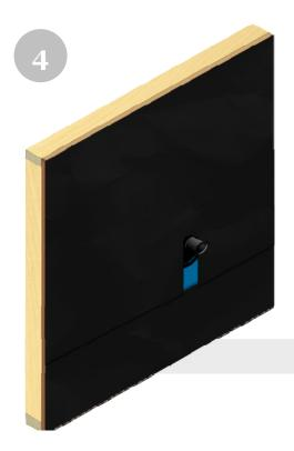
Install the weather resistant barrier carefully cutting an opening around the protruding pipe, over the top of Quickflash® panel using shingle style method extending to the bottom of flashing panel or further down.
