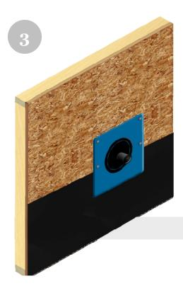
Slide the weather resistant barrier underneath the Quickflash® panel to the bottom of the pipe.
