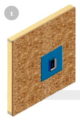
Slide Quickflash® panel onto electrical box firmly pressing panel against the wall or studs.
