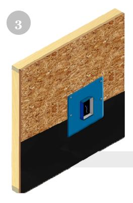
Slide the weather resistant barrier underneath the Quickflash® panel to the bottom of the electrical box.
