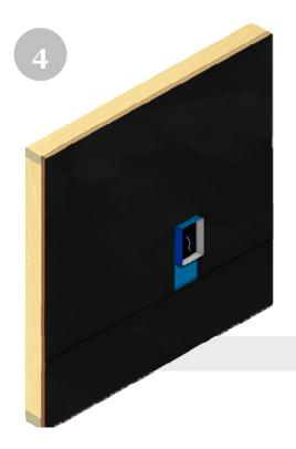
Install the weather resistant barrier carefully cutting an opening around the protruding electrical box, over the top of Quickflash® panel using shingle style method extending to the bottom of flashing panel or further.
