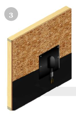
Slide the weather resistant barrier underneath the Quickflash® panel to the bottom of the line-set.
