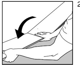
2 Hold the next plank against the first at an angle to the first one and lay it flat on the floor.
