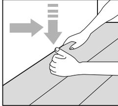
To remove the first row, lift the plank a few centimetres and tap along the joint.
