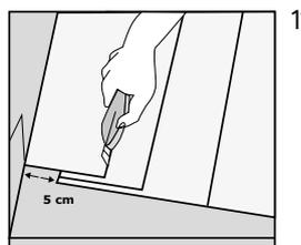
11 Measure and cut the planks in the last row to the correct size.
