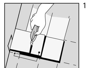
12 The last and first plank can be cut in the correct width. Place the last plank on top of the second to last plank.
