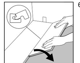
6 Place the first plank of the new row with the tongue side at an angle against the groove side of the plank in the previous row.
