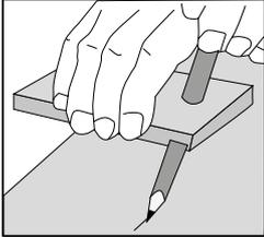
Transfer the shape of the wall to the planks. Do not forget to allow 5mm (0.2") for the expansion gap.
