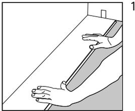
1 Turn the tongue side of the plank facing the wall. Maintain a gap of 5mm (0.2") on the short side.
