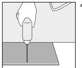
4 Mark where the plank is to be cut and place it on the work surface and cut to size using any kind of saw.
