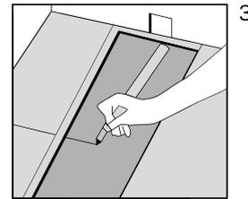
3 Cut the final plank of the first row to the correct length.
