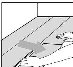
The released plank can then be pulled out. Never bend connected plank backwards, as this will damage the planks.
