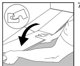
7 Place the short end of the plank at an angle against the previous installed plank and fold down. Ensure that the plank is positioned on the integral locking strip of the plank in the previous row.
