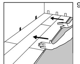
9 Adjust the distance to the wall to 5mm (0.2") when three rows are complete.
