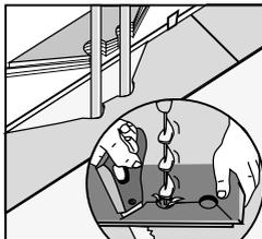
Cut the plank with a 45° angle towards the hole. The cut-off piece is glued in the position again. Cover the hole with a pipe sleeve.
