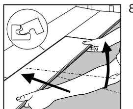
8 Lift the plank (together with the previous one laid in the same row) slightly up (about 30mm (1.2")), push it against the row in front and then put it down.
