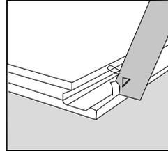
cut away the locking edge and apply Glue (PVA Glue, class D3) on the groove and install the plank
